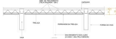
**DETALHE TÍPICO DA ARMADURA DAS TRILHAS**
