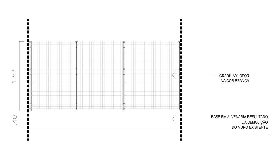
08 DETALHA GRADIL EXTERNO ESCALA — 1:25
