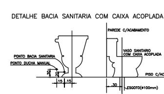
DETALHE BACIA SANITARIA COM CAIXA ACOPLADA
